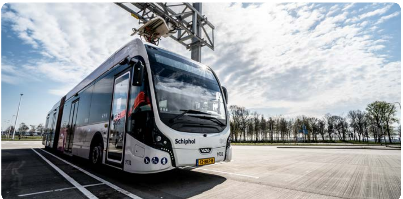
Opportunity-charging AC bus, the Netherlands
